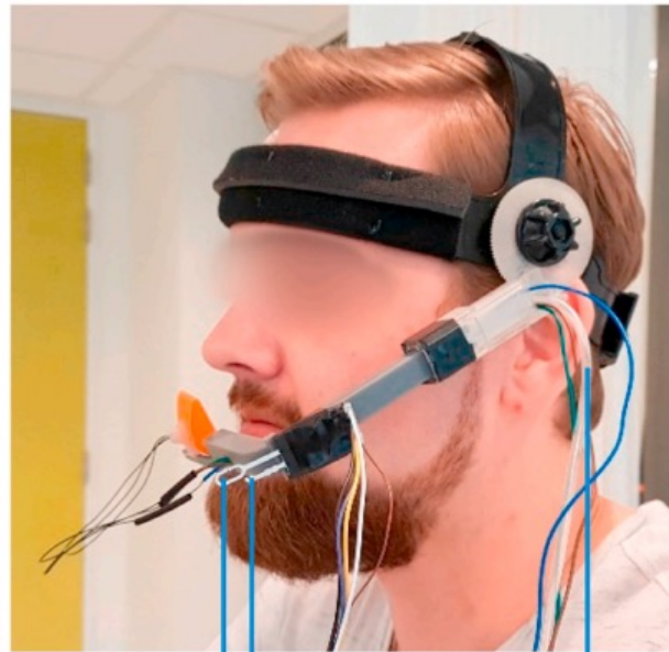
temperature sensor wind sensor sampling tube
